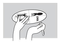
3. Cut the ceiling drywall along the mark you made in Step 2 to create the mounting cutout.
